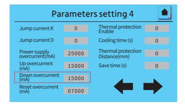
(Please note that if the actuator of the lifting system is ANT-38, the maximum value of Down overcurrent should be 4500 and cannot exceed 4500; if the actuator of the lifting system is ANT-52, the maximum value of Down overcurrent should be 10000 and cannot exceed 10000).
