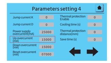
(Please note that if the actuator of the lifting system is ANT-38, the maximum value of Up overcurrent should be 4500 and cannot exceed 4500; if the actuator of the lifting system is ANT-52, the maximum value of Up overcurrent should be 10000 and cannot exceed 10000).
